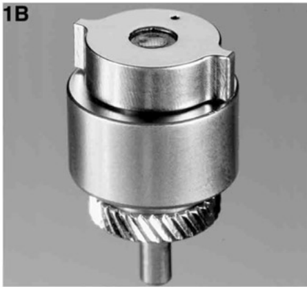
FIGURE 1.—Depiction of the specimen capsule used for imaging of wet samples in scanning electron microscope. A: schematic cross-sectional view of the capsule enclosing a tissue sample. The generally rigid capsule is topped by a window covered by an electron-transparent partition membrane (a). The tissue (b) is held in close contact with the membrane by a spring-supported plunger (c). When placed in the evacuated chamber of the microscope, the tissue is maintained in an aqueous state at atmospheric pressure. A microscopic image is obtained when the scanning electron beam (d) penetrates the partition membrane, interacts with the sample, and backscattered electrons (BSE) (e) are detected by a BSE detector (f). B: external view.
